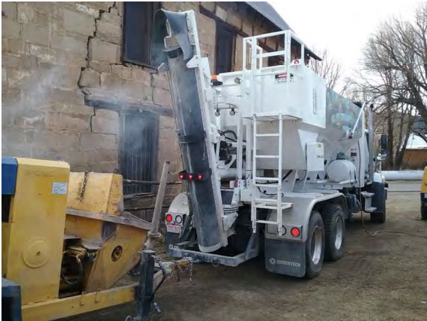
PHOTOGRAPH 13: Grout batch truck
