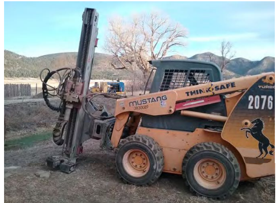
PHOTOGRAPH 8: Skid steer drilling equipment
